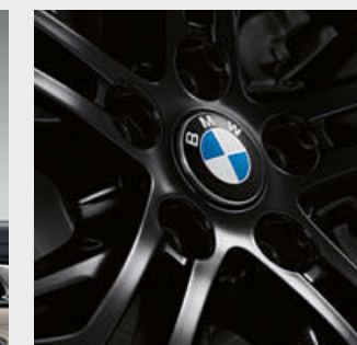
○ The floating hub cap consists of the BMW logo that no longer turns with the wheel but instead remains level.
