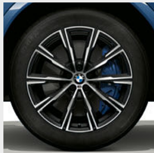
■ 20" M light alloy wheels Star-spoke style 740 M Bicolour Orbit Grey with mixed tyres and runflat tyres*, gloss-lathed, front 9J x 20 with 275/45 R20 tyres, rear 10.5J x 20 with 305/40 R20 tyres. 2
