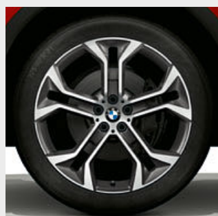
□ 21" light alloy wheels Y-spoke style 744 Bicolour Orbit Grey with mixed tyres and runflat tyres*, gloss-lathed, front 9.5J x 21 with 275/40 R21 tyres, rear 10.5J x 21 with 315/35 R21 tyres.
